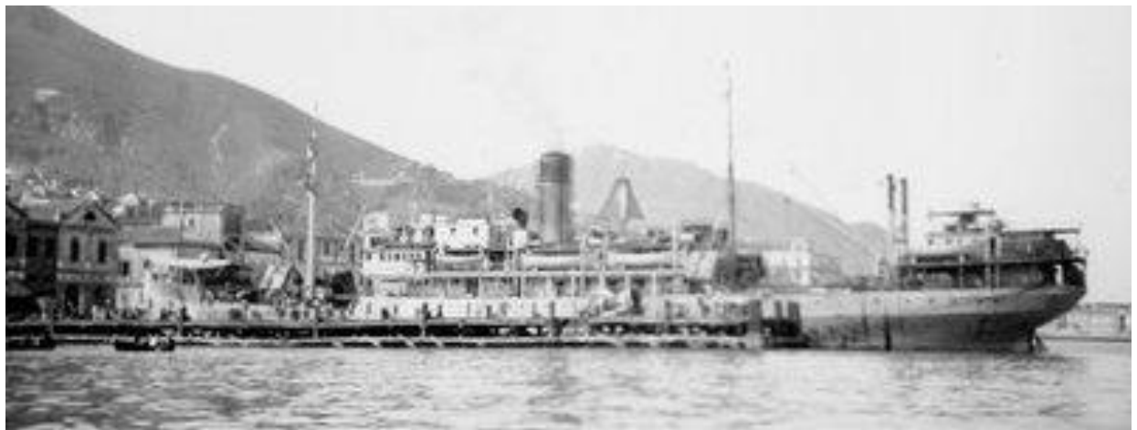
YUEN SANG in 1945/46 with superstructure enclosed forward (NMM).
