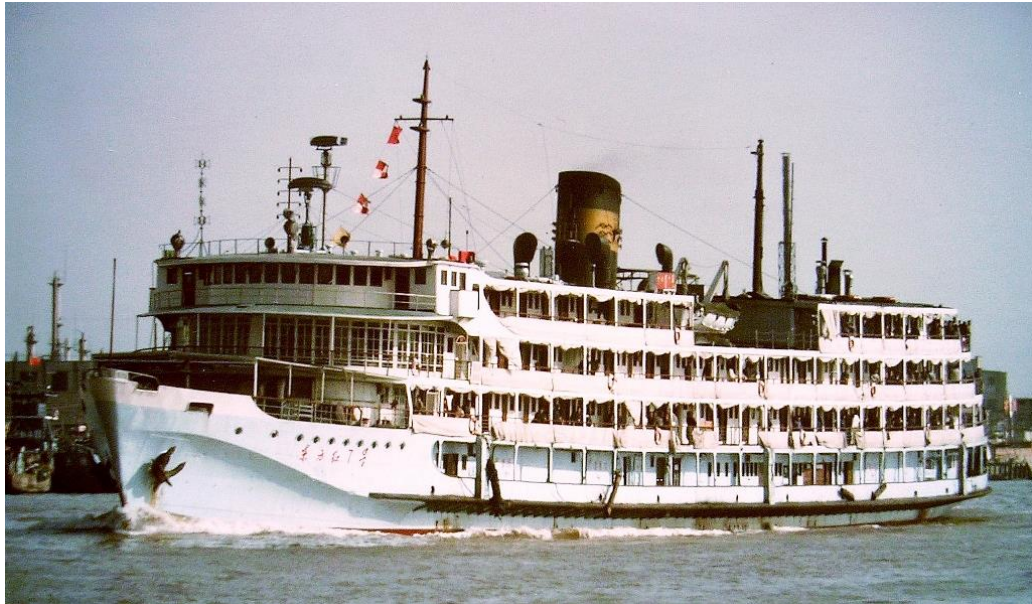
DONG FANG HONG 7 ex TUCK WO at Shanghai 1977-79, new radar and searchlights, shortened masts (Ted Scull*).
