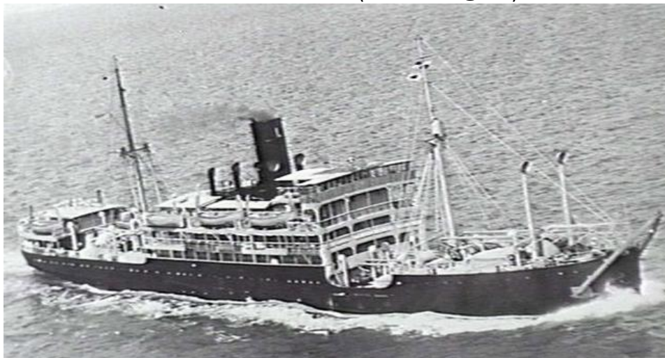
TAIPIING on 21 Dec. 1940 with a frame for paravane gear fitted at the bow (AWM303999)
