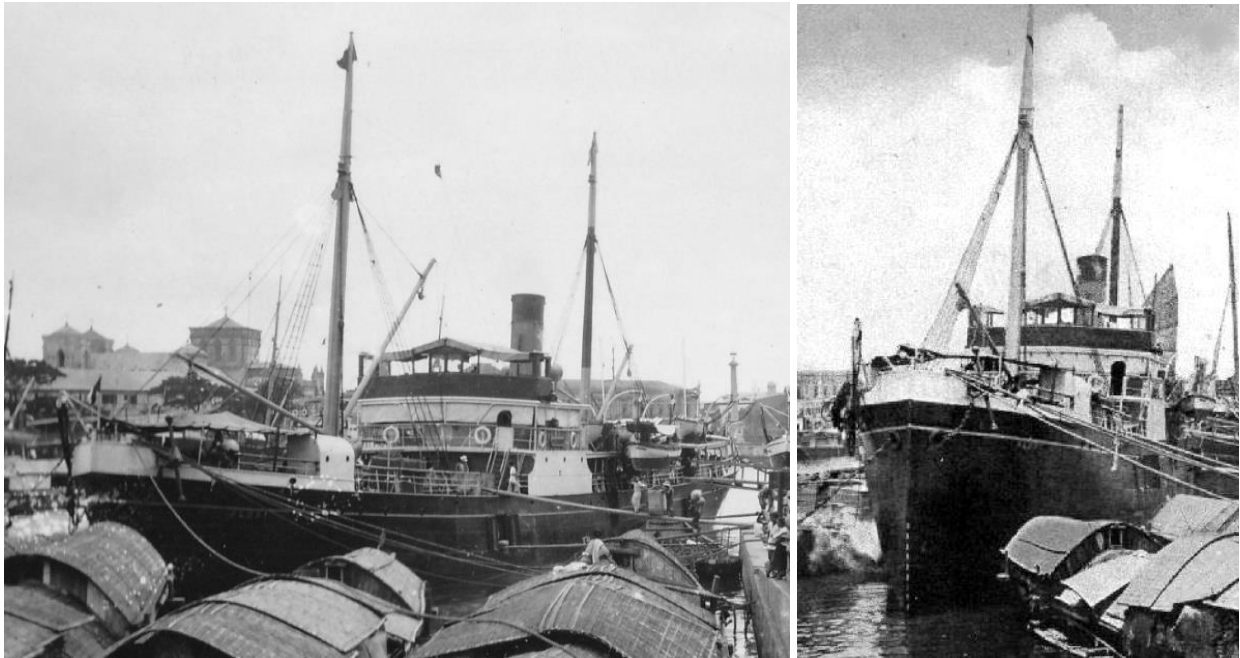
Updated JOSEFINA (I), bridge more substantial and one deck higher (l. John Tewell; r. postcard).
