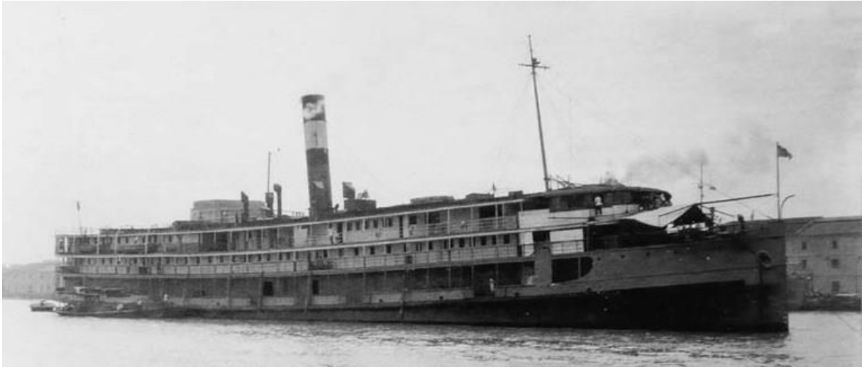
KIANG HSIN reconstructed postwar with rounded bridge and no mainmast (Yao Kaiyang coll.).
