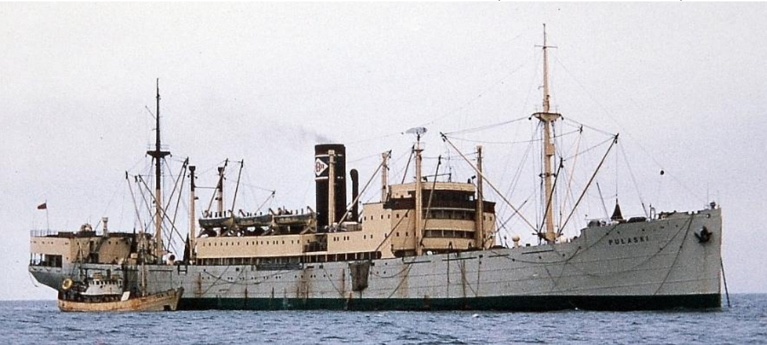
PULASKI post-1960 rebuilt for PPDiUR as fisheries mother ship with extra accommodation on boat deck and aft (coll. H. Stott).
