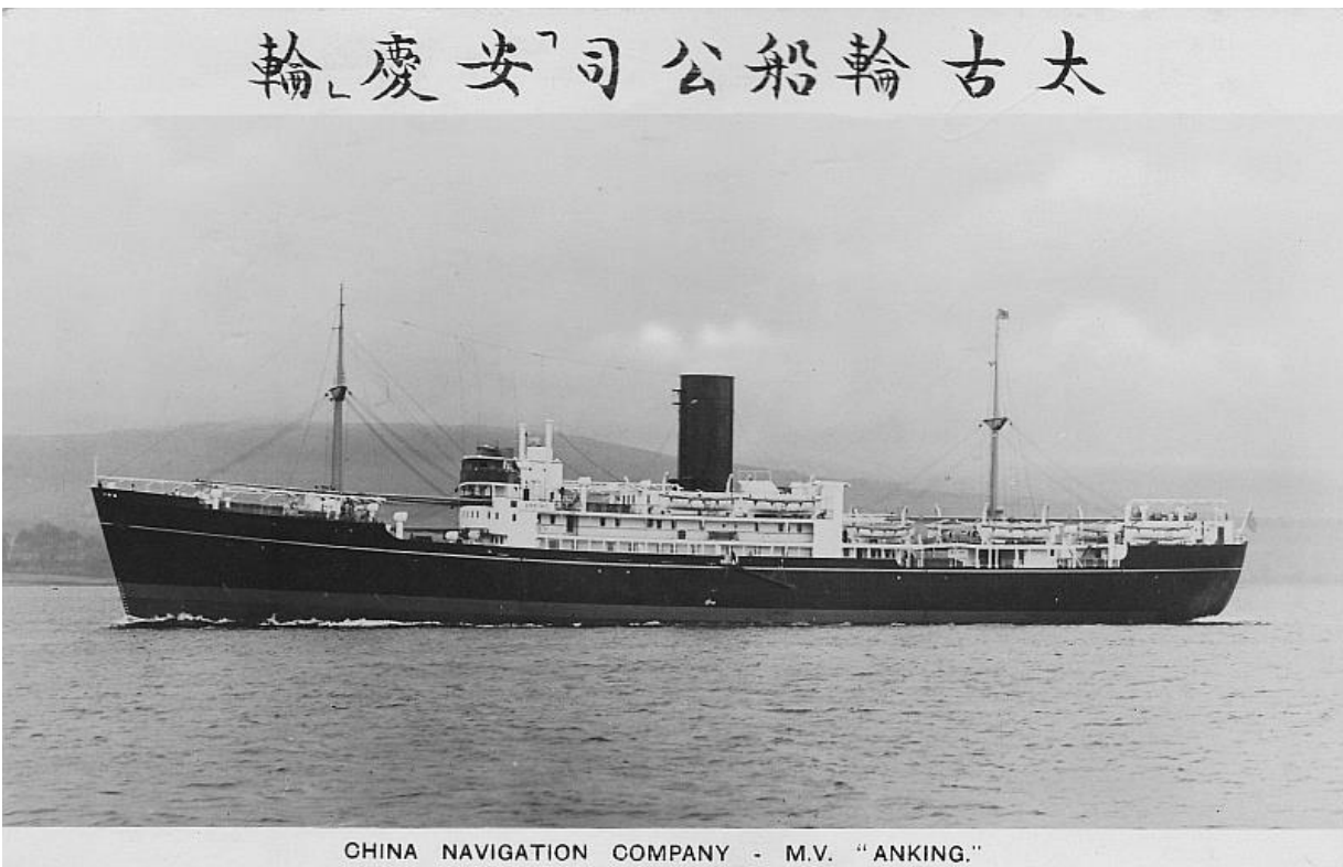
Official CNCo postcard of ANKING on trials in the Clyde, December 1949. The wide plating at either end of the central accommodation block is part of the anti-piracy grilles (coll. H. Dick).
