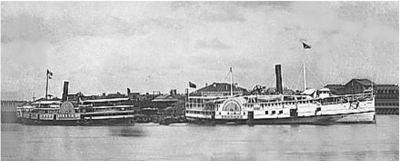
CNC's buff-painted iron-hulled ICHANG (l.) with refitted wooden-hulled KINSHAN (r.) at Canton. KINSHAN's iron hog bar, strengthening the hull longitudinally, is visible above the deck (Internet).
