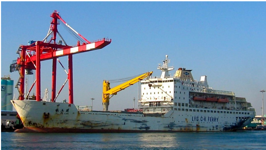
ZI YU LAN at Incheon, hull with rubbing marks from the locks there (Jim Shaw).
