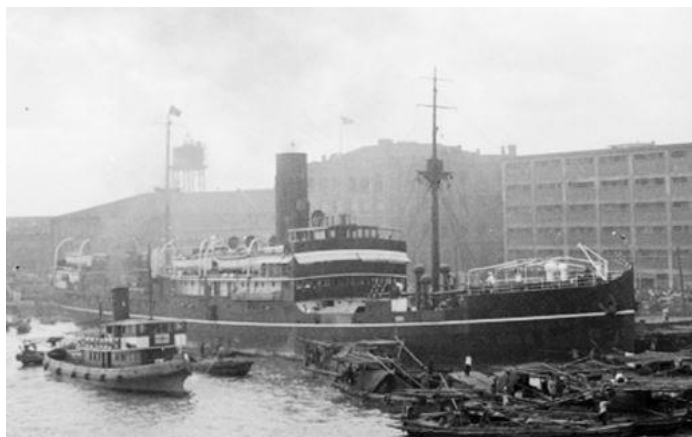
HANYANG at French Bund, Shanghai, 1940. Ventilators in front of funnel soon relocated behind, lower ventilators heightened (Warren Swire/UoB Sw08-181).
