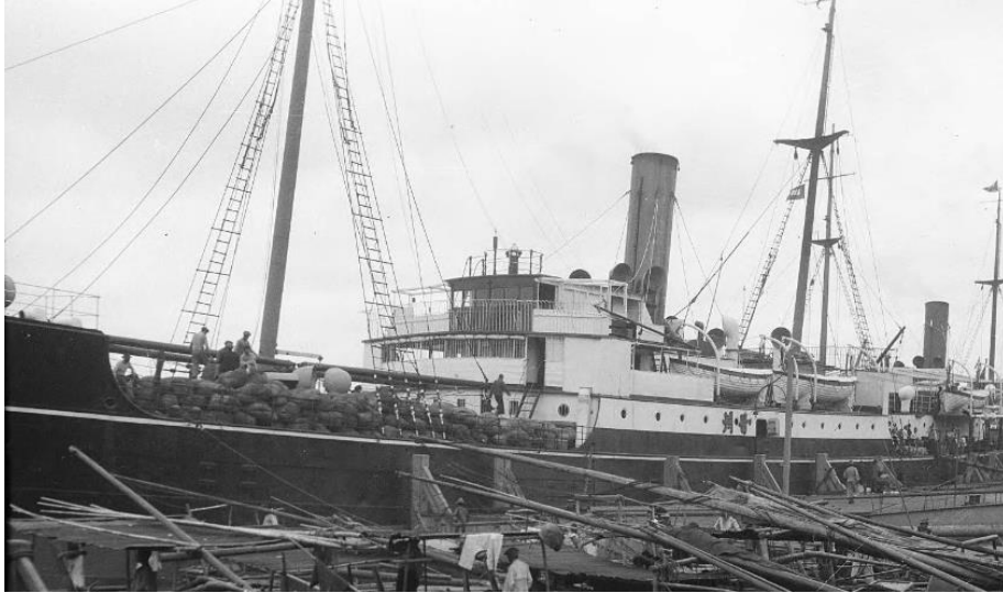
KANCHOW at Shanghai 1931-32. The 'Chow' class of six 267' ships is distinguished by a shorter No.3 hatch and a large curved tree on the mainmast (Robert Larimore Pendleton pe001931/UWM Libraries).
