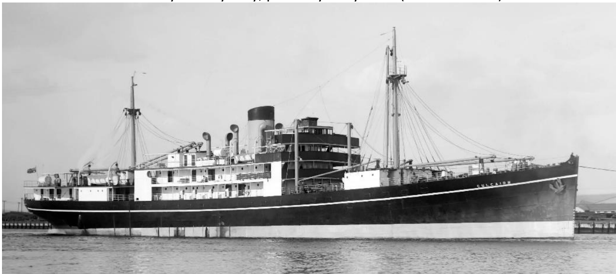
Refitted CULCAIRN ex-ANSHUN at Melbourne, still with China coast mast housings and remnants of anti-piracy plating (AC. Green/SLV).
