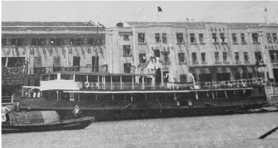
Assumed TSZPEH alongside at Ningpo 1934 with bridge structure extended aft and stern plated in around the upper deck (Wang Zhi-Xiang/Ningbo Museum).
