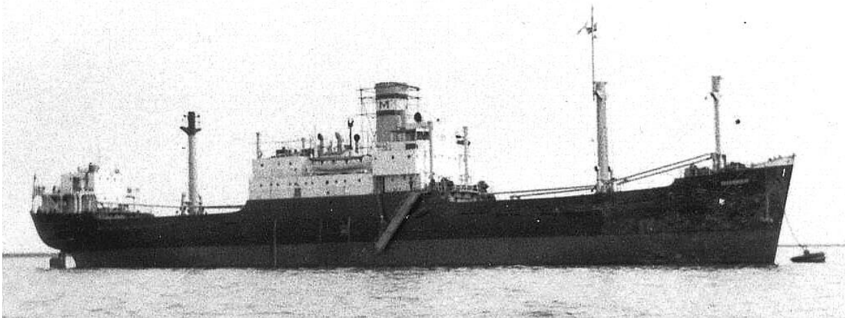
TEES BREEZE with scaffold around a bigger funnel replacing the original stovepipe (coll. S. Kentwell*)
