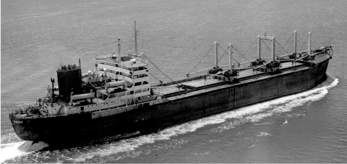
COSMO TRADER (III) as WINFIELD TRADER showing bridge structure repositioned aft and four long hatches in the well (H. Dick collection).
