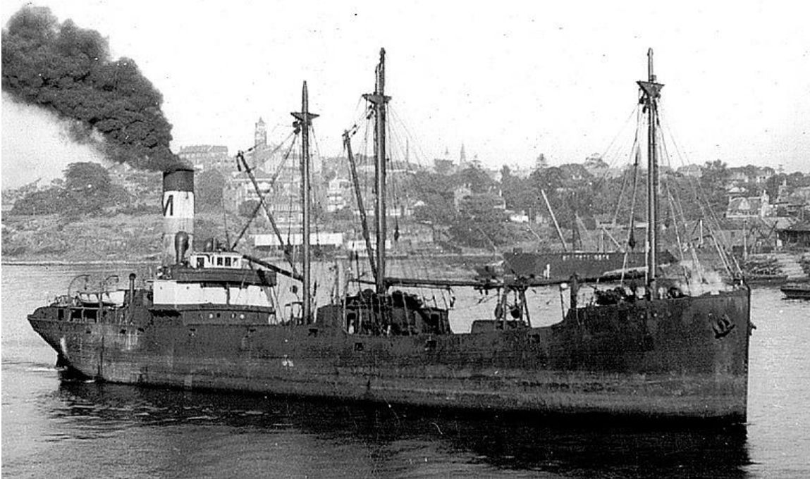
R.W. Miller's coal-burning collier CANOPUS departing Sydney for Newcastle, coal grabs stowed for sea (H. Dick collection).
