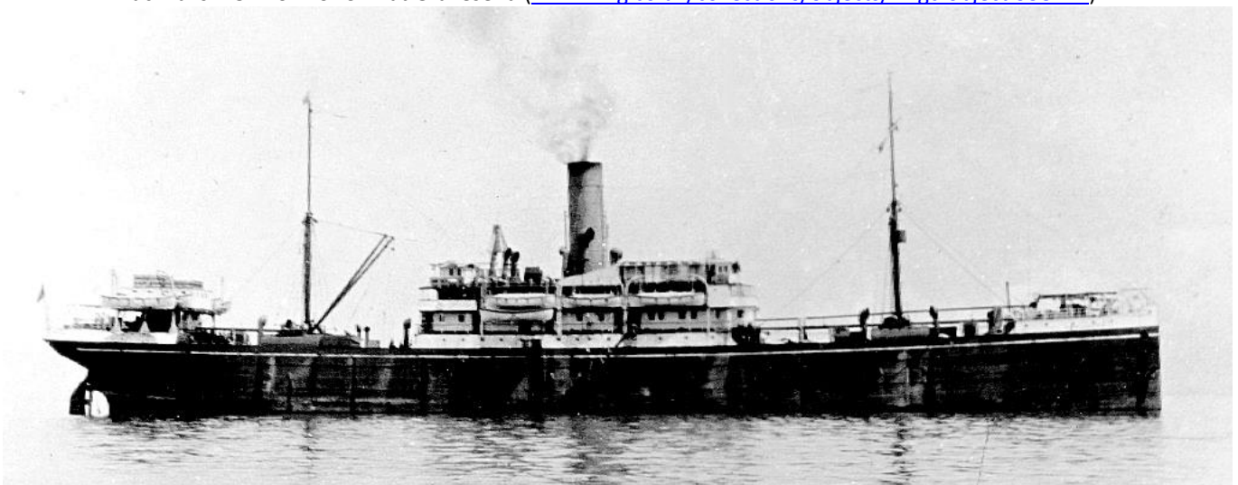
Nemazee's GORJISTAN at Tanjung Priok (Jakarta) in mid-1920s. More ventilators and side housings added by Bank Line for tweendeck passengers, also taller funnel (KPM archive, Alg. Rijksarchief).
