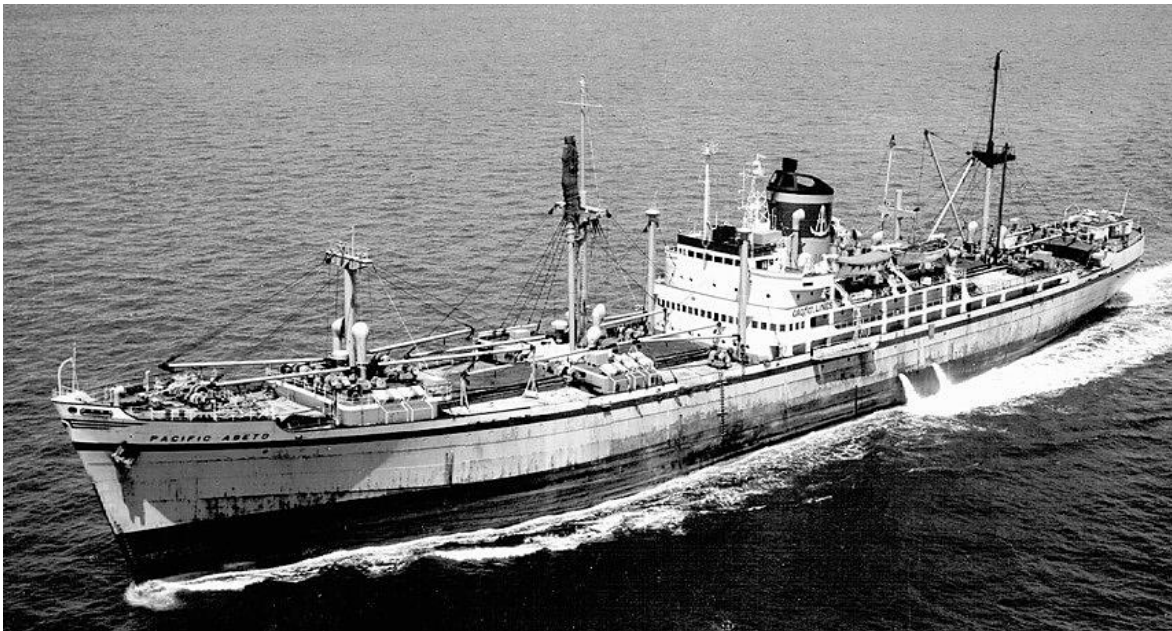
PACIFIC ABETO light-ship in Straits of Malacca, no passengers but life rafts at masts. Accommodation extended aft at No. 4 hatch and row of 'tweendeck portholes visible beneath green hull band (Peter Foxley).
