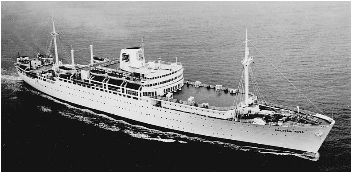
All-white MALAYSIA RAYA in Malacca Strait. No. 2 (with well) and No. 3 hatches suppressed and accommodation extended to the foremast (Peter Foxley).
