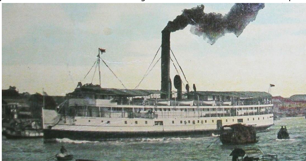
CHARLES HARDOUIN (from a postcard). Large ventilators abaft funnel are an identification marker.
