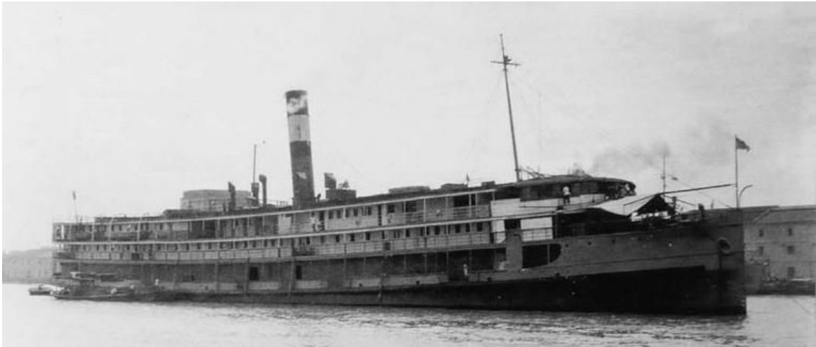
KIANG HSIN reconstructed postwar with rounded bridge and no mainmast (coll. Yao Kai-yang).
