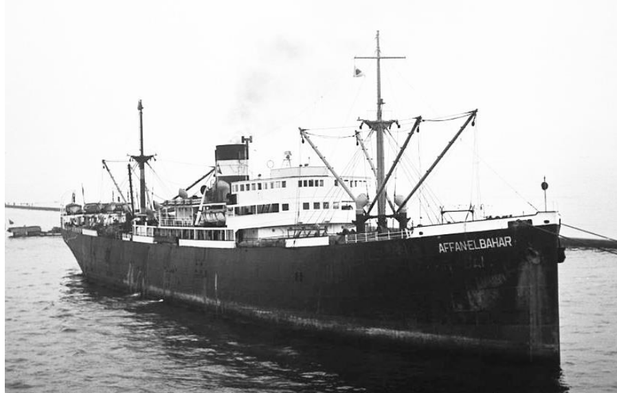
AFFAN-EL-BAHAR ex HONGKONG FIR at Kobe, Nov. 1964. Temporary mast housings now removed, boat moved forward, extra boats at the stern (Dr. George Wilson).
