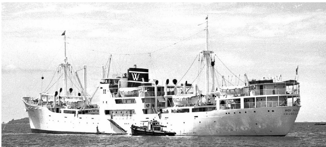
Ca.1961 improved boats and more prominent ventilators fore and aft (R. Gabriel/H. Dick).
