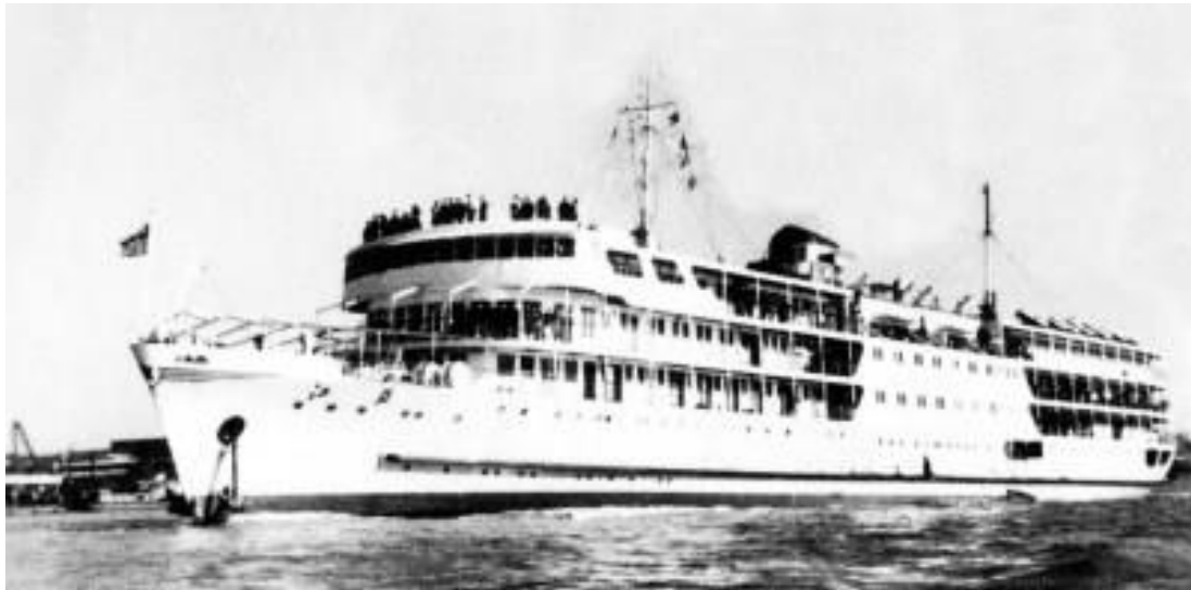
JIANG YA, was raised in two sections and rebuilt, re-entering service on the Yangtse in 1959 ( http://ayuczds.blog.163.com/blog/static/22154207320135173213612/ ).
