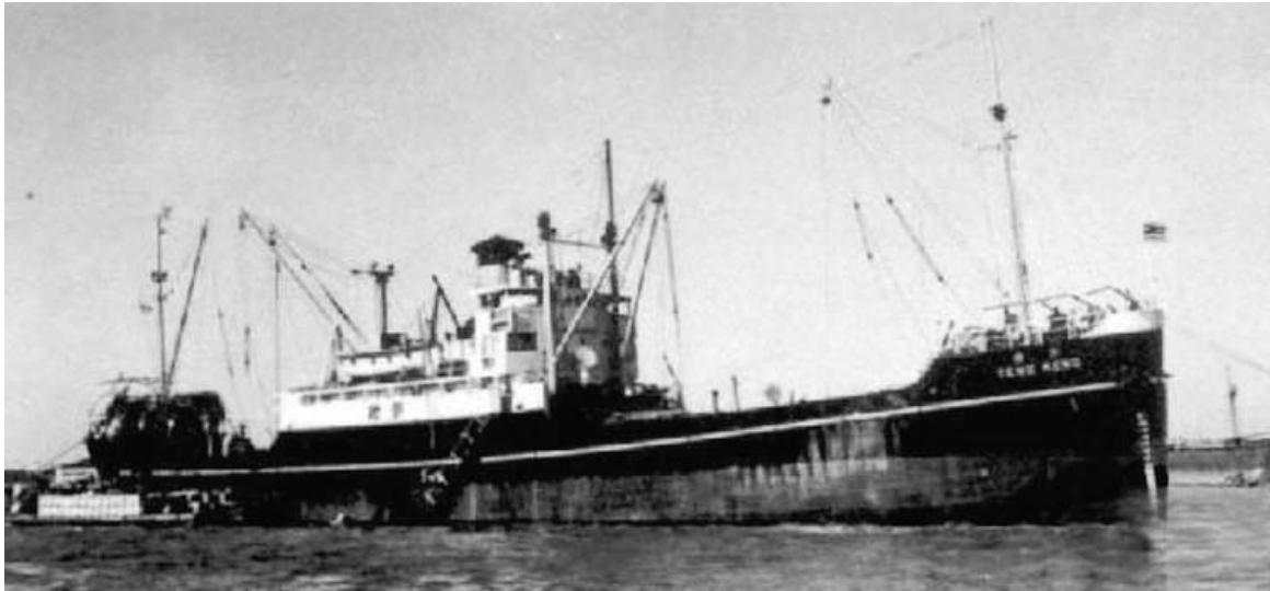
TENG KENG was a standard N3 'Jeep' (I Wen Hua Pao July 1948).
