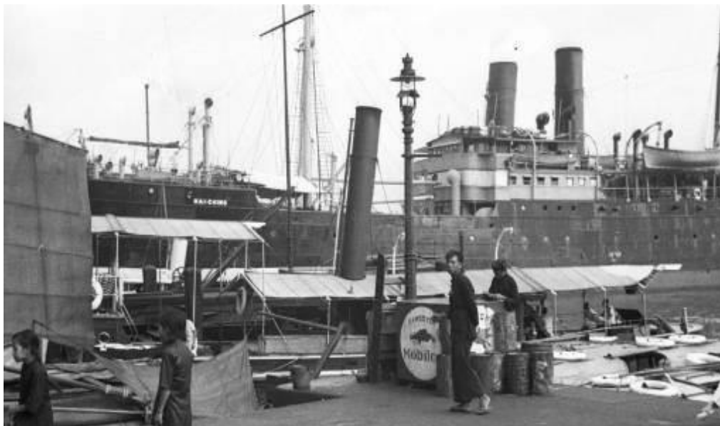
HAICHING at Hong Kong, probably on 16/9/40, after further reconstruction with more enclosed superstructure, upright masts and funnel, and kingposts on fo'c'sle. SEISTAN behind and small DSSC tender in foreground (Harrison Forman/University of Wisconsin-Milwaukee Libraries).
