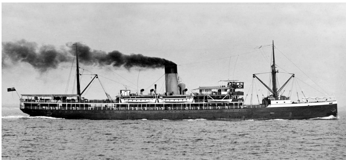
HAI LOONG before acquisition as Adelaide S.S. Co. MORIALTA. As built with low fo'c'sle and flying bridge plus radio aerials (A.C. Green/State Library of Victoria).
