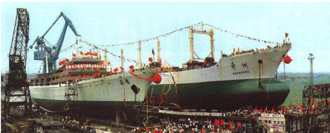
CHANG Zi on launch day, indicating forward kingposts, mainmast and crane aft. Bulk carrier alongside is SHENZHOU.
