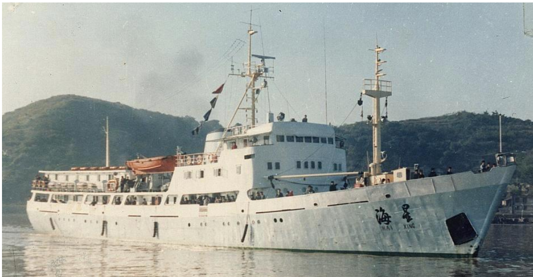
HAI XING as later modified with deckhouse aft (Xinhua).
