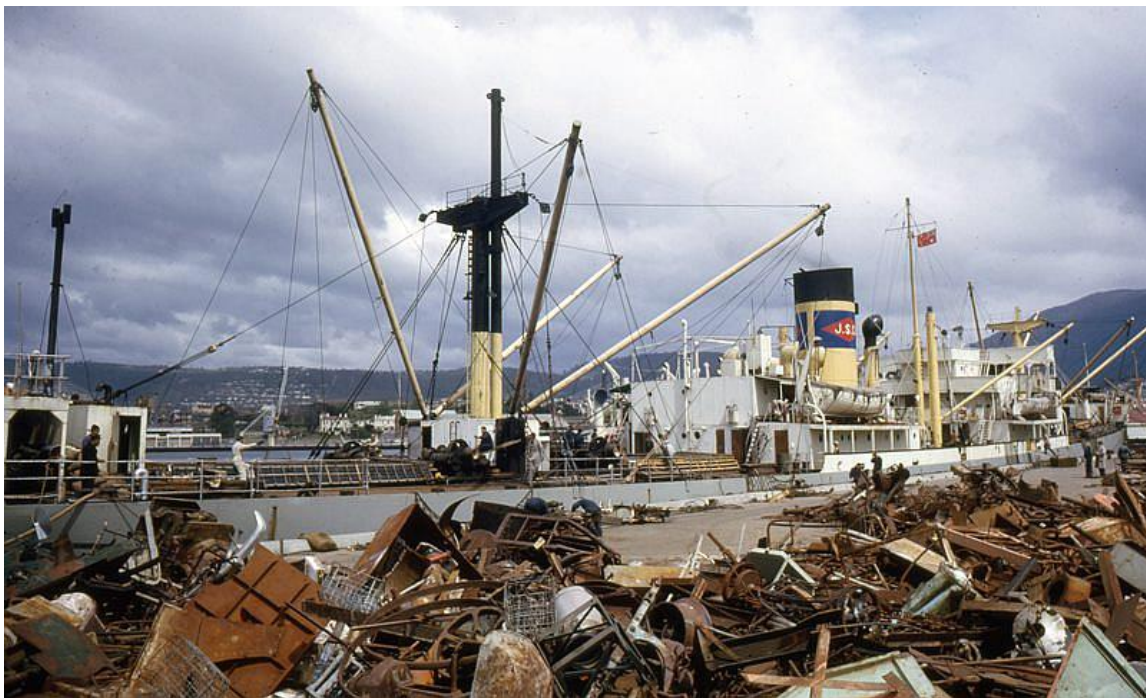
SHUN TAI at Hobart, October 1964, loading scrap dumped onto the wharf in bits and pieces and lifted by grabs. The ship is well down after prior loading at Sydney and Melbourne. Still in wartime rig (no topmasts) but a tall stovepipe added aft for the Chinese crew's galley (G. Allan/R. Cox).
