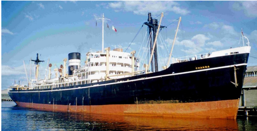
PRECIOUS PEARL as BI's CHANDA at Hobart, 1958/59, wartime rig with signal mast in place of topmasts (unknown/NAA).
